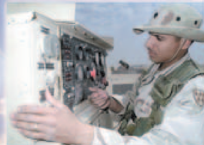
Launcher crew member Spc. Miguel Alvarez confirms generator volts and Hertz are at optimum performance for Patriot missile operation.
